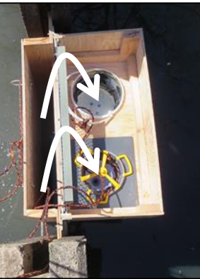
An airlift pump chamber was installed to circulate water from Cell 3 to Cell 4 through zooplankton collection nets.
